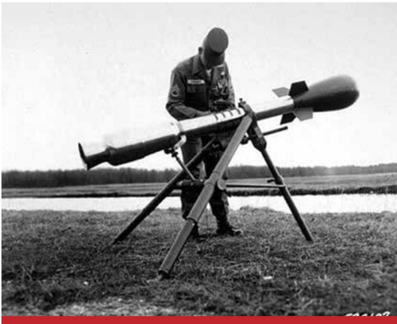
Fig. 1: Davy Crockett nuclear recoilless gun
